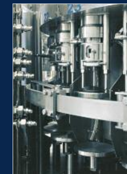
Valvola isobarica meccanica Mechanic isobaric filling valve
