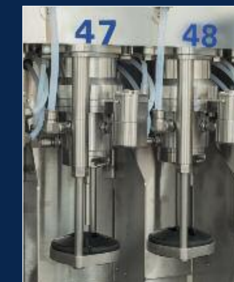
Valvola isobarica elettronica elettropneumatica Electronic-electropneumatic isobaric filling valve
